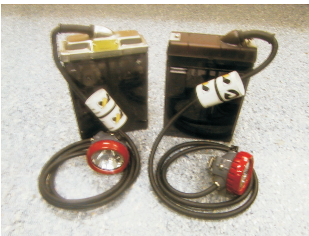
FIG 2 - LAMPS type II tags mounted on GT2 battery cord (left) and GT5 battery cord (right).
